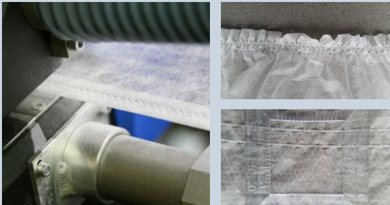
Details of process and samples with glueless elastic application
