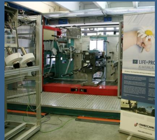
The Fameccanica lab test stand for glueless elastic strands application
