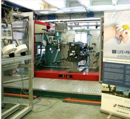
The lab test stand for GLUELESS™ elastic strands application
